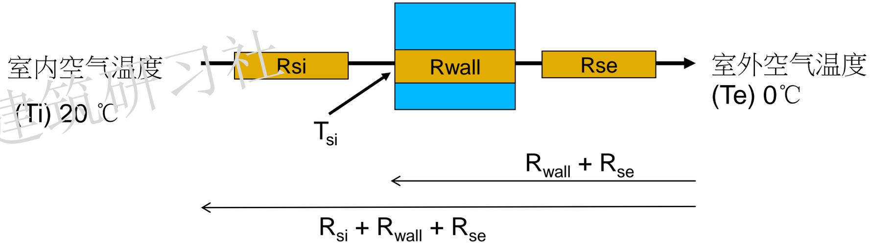
$$F_{rsi} = (R_{wall} + R_{se}) / (R_{si} + R_{wall} + R_{se})$$
